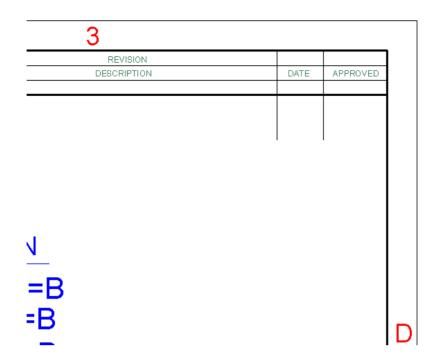
The process of zoning in a drawing is referring to finding the location of a specific part, usually used in an assembly drawing where there are many parts. This process is kind like reading a map.
