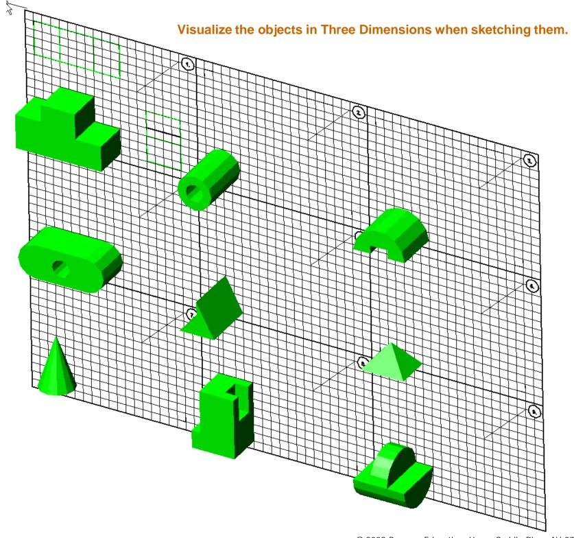
On the grid sheet provided, sketch the Front, Top and Right side views of the objects shown below. Begin views in the corners shown in the grid.
