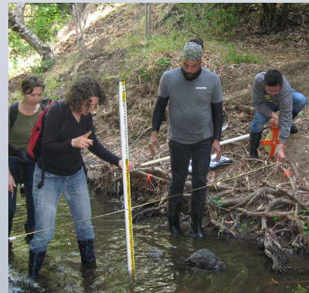
Using a stadia to measure the depth of flood-prone bank during a riverine CRAM session.
