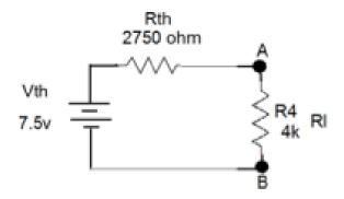
13. Calculate the total load current & load voltage.
