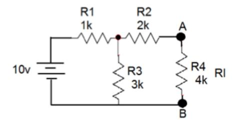
Open the 4kΩ load resistor
