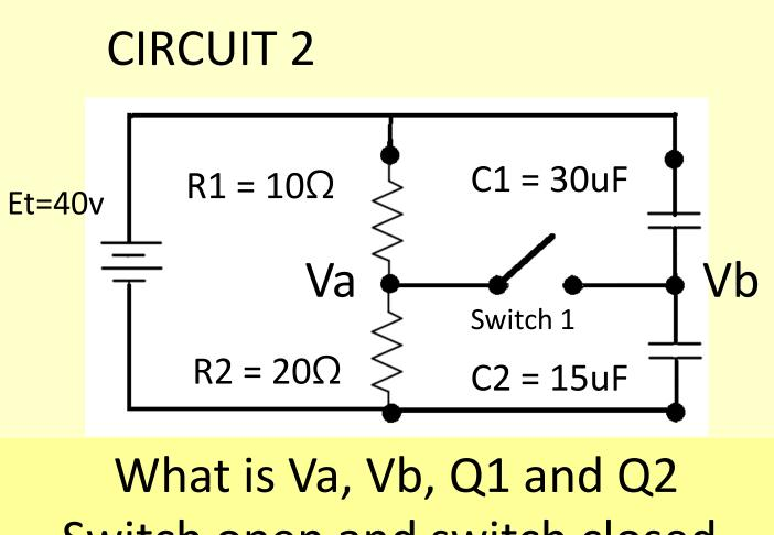
Switch open and switch closed.
