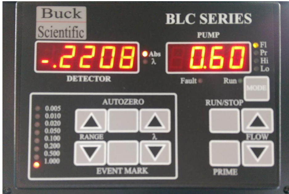
Figure 2. HPLC Front Panel
