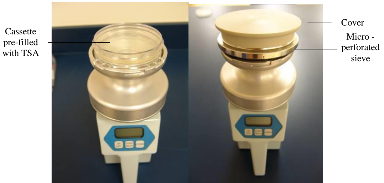
Figure 3: Diagram of the M Air T Millipore Air Tester with Installed Cassette, Micro Perforated Sieve and Cap
