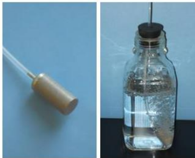
Figure 2. Porous Metal Sparger
