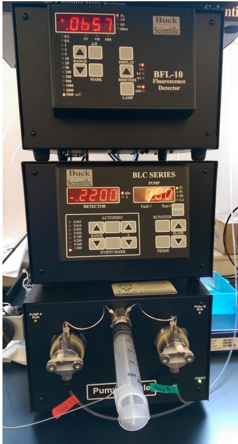
Figure 1. Buck Scientific BLC-20G HPLC System with Pumps and Detectors
