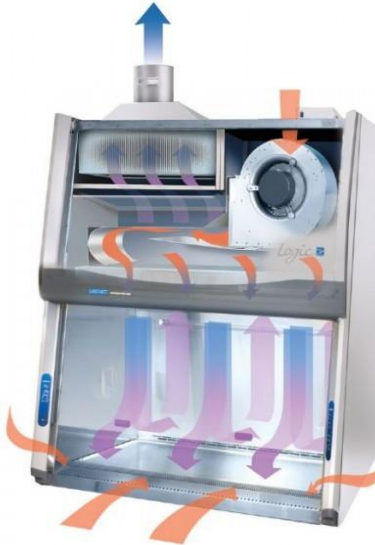
Figure 3: Air Flow Diagram
