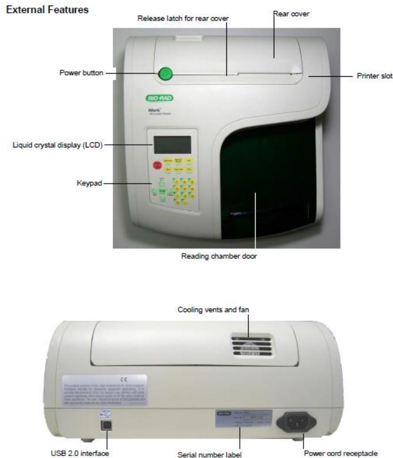
Figure 1. External Features of Bio Rad iMark Microplate Absorbance Reader
