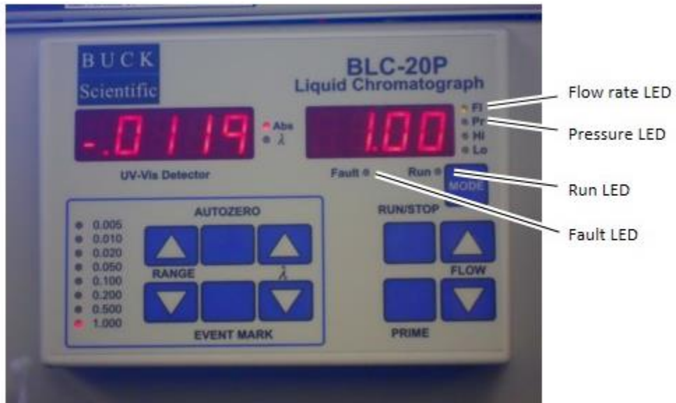
Figure 2. HPLC Front Panel
