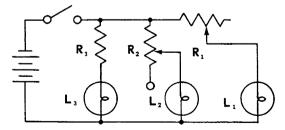
113. When connected in a circuit, a rheostat is readily distinguishable from a potentiometer because a rheostat uses \_\_\_\_\_\_\_ connections, and a potentiometer uses \_\_\_\_\_\_ connections.
