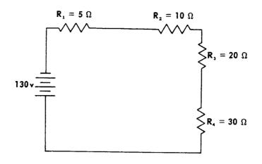
The total resistance is \_\_\_\_\_ ohms.
