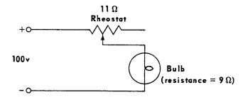
The rheostat can be varied from 0 ohms to \_\_\_\_\_\_ ohms.
