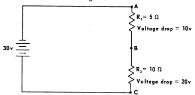
The ratio of the resistances is 5/10, or 1/2. The ratio of the voltage drops across these resistors is
