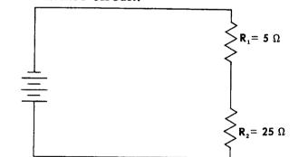
The voltage drop across  $R_1$  is 20 volts. The voltage drop across  $R_2$  must be volts. (Resistance ratio = 5/25 = 1/5.)
