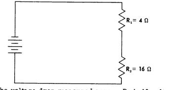
If the voltage drop measured across  $R_1$  is 10 volts, the voltage drop across  $R_2$  is \_\_\_\_\_\_ volts.
