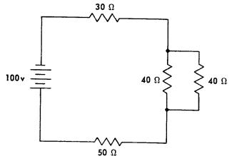
The two 40-ohm resistors in parallel are equal to one \_\_\_\_\_\_\_-ohm resistor.
