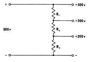
103. This circuit can be used as a voltage divider.
