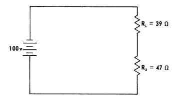
The voltage drop across  $R_1$ , to two decimal places, is \_\_\_\_\_\_ volts. The voltage drop across  $R_2$ , to two decimal places, is \_\_\_\_\_\_ volts.
