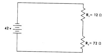
The total resistance is \_\_\_\_\_\_ ohms. The l2-ohm resistor is what fraction of the total resistance?
