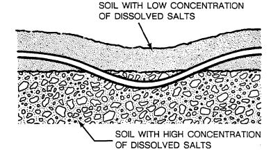
The area of pipe that is in contact with a higher salt concentration is highly corrosive.
