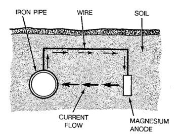
When connecting a magnesium anode to an iron pipe, the pipe will (corrode / be protected).
