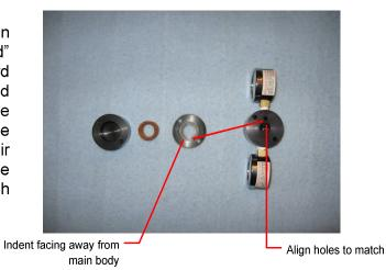
Make sure that the "nut" side of the diaphragm is towards the main body and that the "bullet" protrudes through the outer section of the bottom plate. The stem side of the spring will mate into the "nut" portion. Reinstall bolts and tighten. Snap pilot assembly is now complete.
