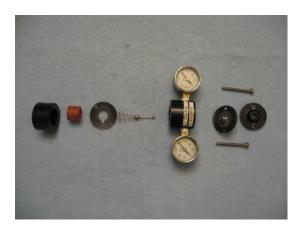
When placing the bottom section together, ensure that the "indented" side of the rubber is facing toward the cavity of the upper section and not against the main body. Align the notch in the rubber to line up with the hole in the main body. Place the air screen and spring end inside the upper section and fit stem through main body.
