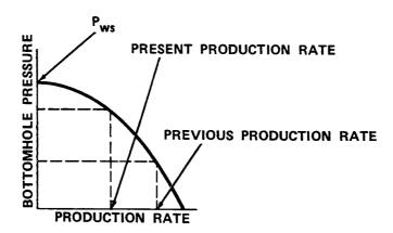
The producing bottomhole pressure is ( higher / lower ) than before.
