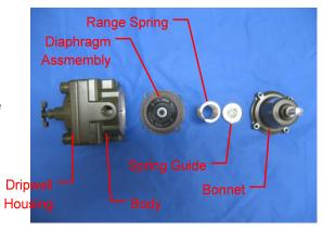
Clean the dripwell housing with fresh water. Lubricate the springs and components with grease.
