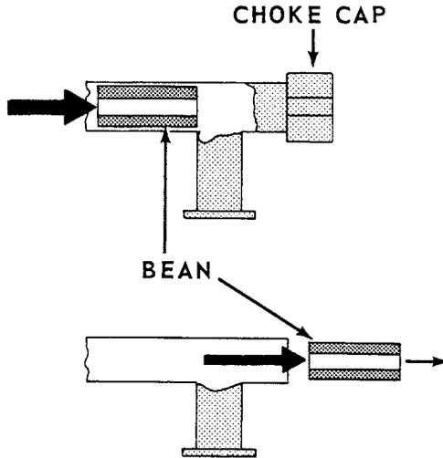
When the choke cap is removed, the \_\_\_\_\_ will shoot out of the tee.
