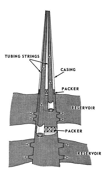
Then fluid from the lower reservoir is directed into the \_\_\_\_\_ by a packer.
