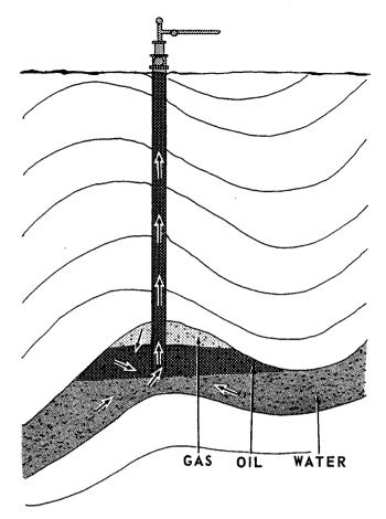
For optimum recovery, you want to draw fluid from (all three fluid layers/only the layer of oil).
