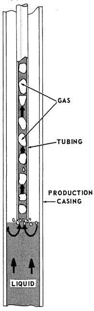
Then the high-pressure gas from the annulus blows around into the \_\_\_\_\_.
