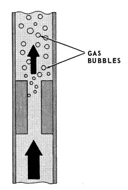
The reduction in pressure often allows \_\_\_\_\_\_ to expand downstream from the choke.
