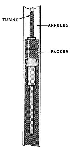
Packers prevent fluid from entering the \_\_\_\_\_.
