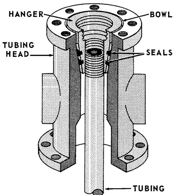
The tubing head is flanged, studded, or threaded onto the uppermost \_\_\_\_\_.
