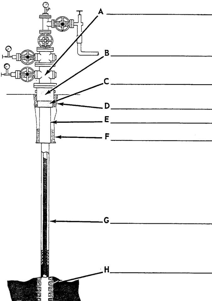
29. You can calculate the number of casing strings in the well-bore by counting the casing heads.
