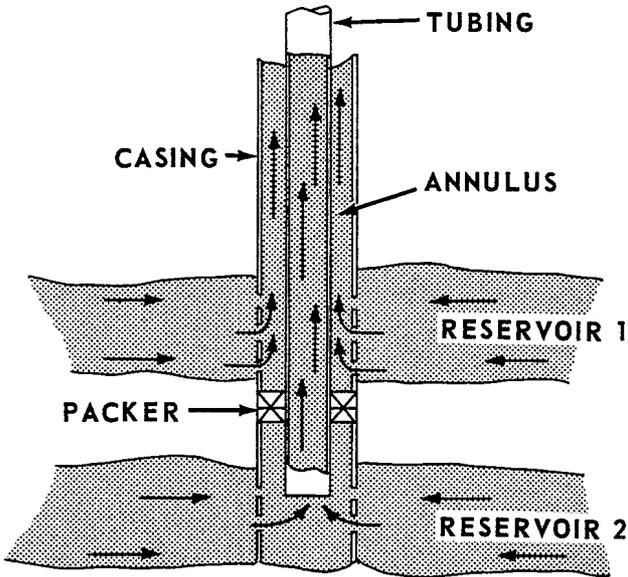
At one time, a multiple-completion well produces from (only one/more than one) formation.
