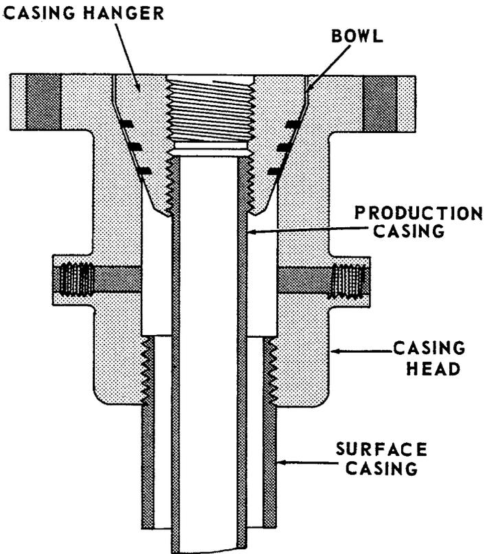
The casing head has a \_\_\_\_\_ which supports the casing \_\_\_\_\_.
