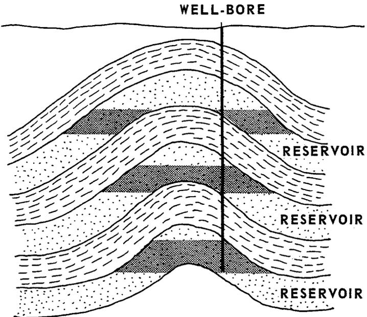
Then the same well-bore cuts through more than one \_\_\_\_\_.
