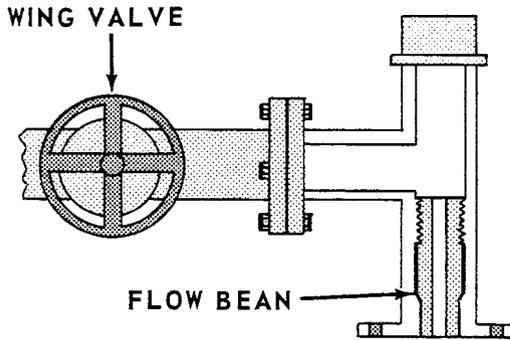
The orifice in a positive choke is called a flow \_\_\_\_\_.
