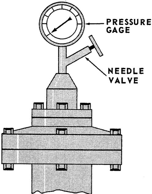
The pressure gage registers the pressure in the (tubing/annulus).
