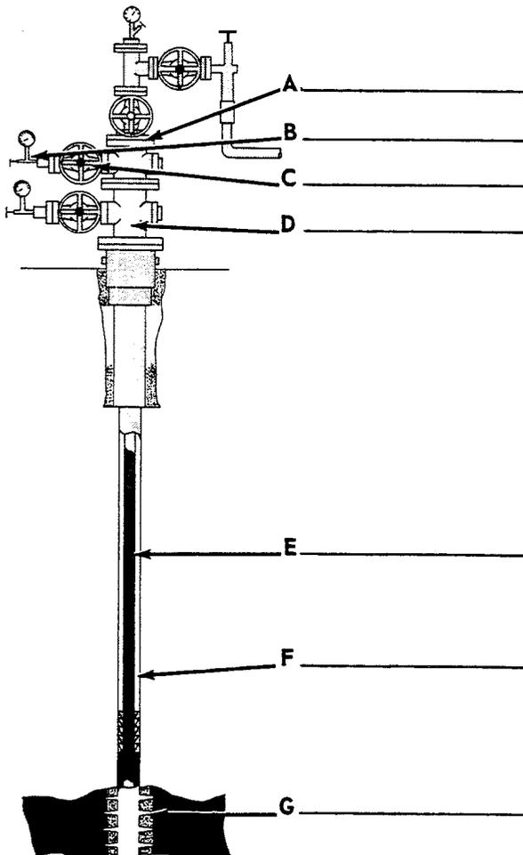
49. In some wells, the casing heads and tubing head are all in one piece of equipment.
