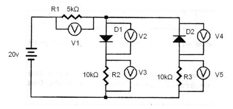
Step 11. Predict and measure the voltages. Place the measured values into the table.
