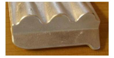
Hot tear – due to difference in cooling rates between thin and thick sections (a crack formed while the casting is cooling)
