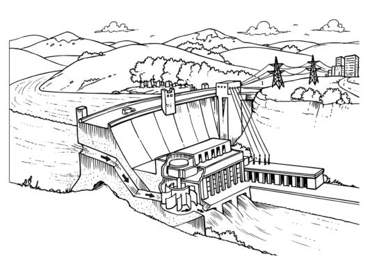
In hydroelectric power plants, the **mechanical energy** to rotate the generator comes from the force of **falling water** pushing against the blades of a water turbine.
