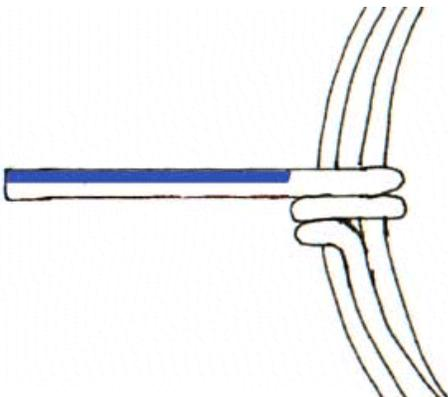
Scrape the insulation off the top side of both wires. In this picture, bare wire is blue.
