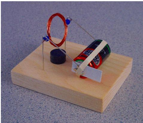
8) If your motor is especially well balanced the motor might start spinning right away. If not, give the coil a spin in either direction. The motor will either speed up or slow down and reverse direction.
