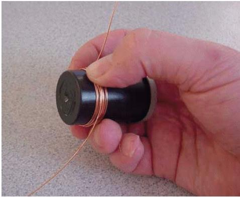
3) Next, hold the coil so it doesn't unwind and wrap about three turns of the bent end of the wire tightly around the coil. Then wrap the free end several turns around the other side of the coil. The balance of the coil is important so try to get the two wire ends on directly opposite sides of the coil. Use wire cutters to trim the wire ends approximately  $\frac{5}{8}$ " long
