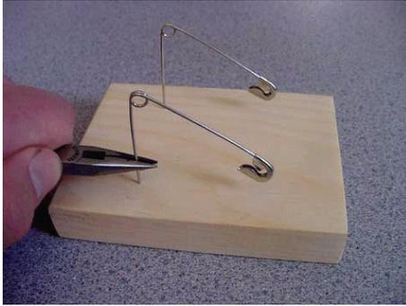
6) Slip a bead over each end of the wires on the coil and gently spread the safety pins apart and slip the wire ends into the loops of the safety pins. Adjust the balance of the coil by bending the wire ends or sliding the wrapped ends up or down slightly. Once adjusted the coil should spin freely when you give it a spin. If the coil won't spin freely, the motor won't work.
