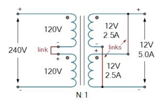
3) What is phase relationship between the primary and the secondary of the transformer shown below?
