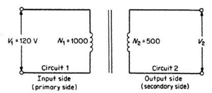
2) What is the turns ratio for the transformer shown?
