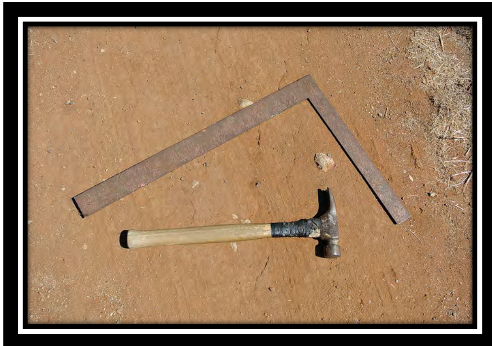
Figure 9 – THOR's hammer and framing square DSC_0544 (el cajon yacht club, CC BY – 2.0)
