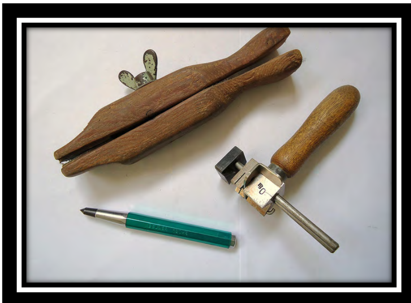
Figure 22 – My Studio (Mauro Careb, CC BY – 2.0) Image: Ring clamp, center punch, and jog for tube cutting
