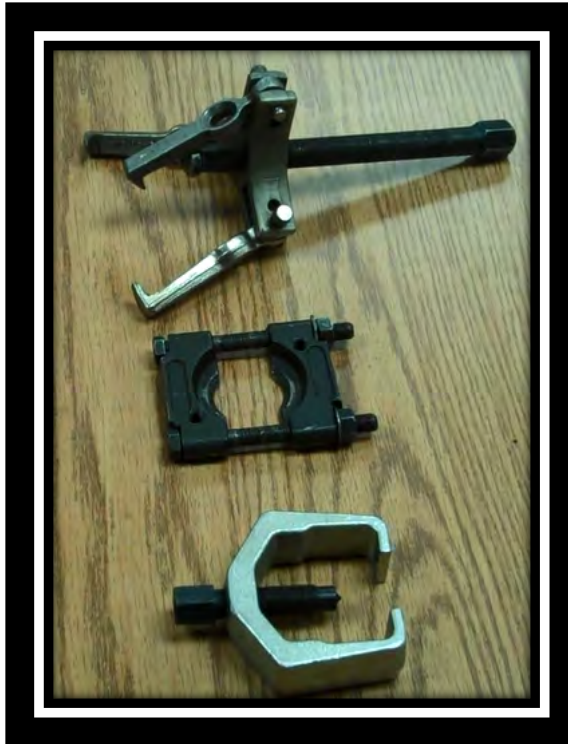
Video 9 – Pullers (York Technical College, CC BY – 2.0) For a transcript of this video, please click on transcript .
