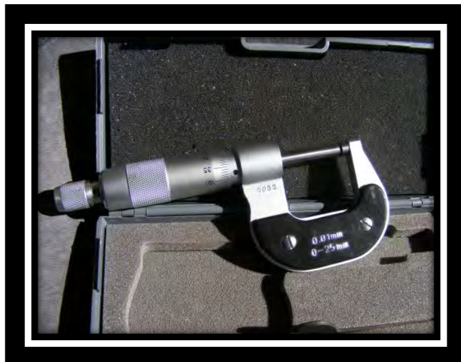
Figure 6 – External - Micrometer – Screw – Gauge_23114 – 480 x 360 (Emillan Robert Vicol, CC BY 2.0) Image: External Micrometer
