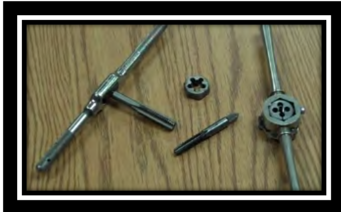
Video 3 – Taps and Dies (York Technical College, CC BY) For a transcript of this video, please click on transcript .
