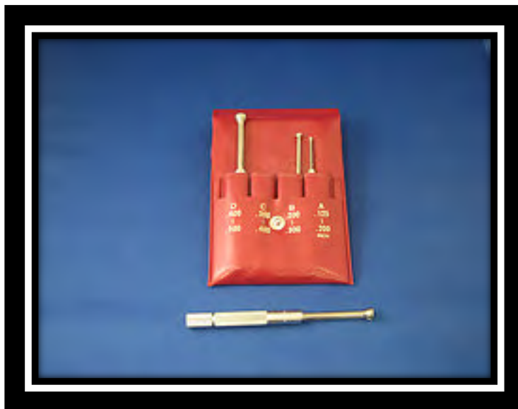
Figure 7 – small hole gauge [gauge] (Connie Posites, CC SA 2.0) Image: Small hole gauge set
