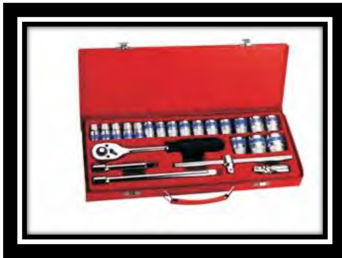
Figure 12 - socket set (Jonathon Stewart, CC BY – NC – ND 2.0) Image: socket set with various size sockets, ratchet, and extender bars.
