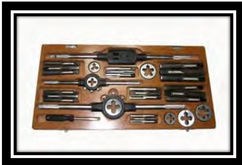
Figure 5 – tap die (Jonathan Stewart, CC BY – NC- ND 2.0) Image: Tap and Die Set
