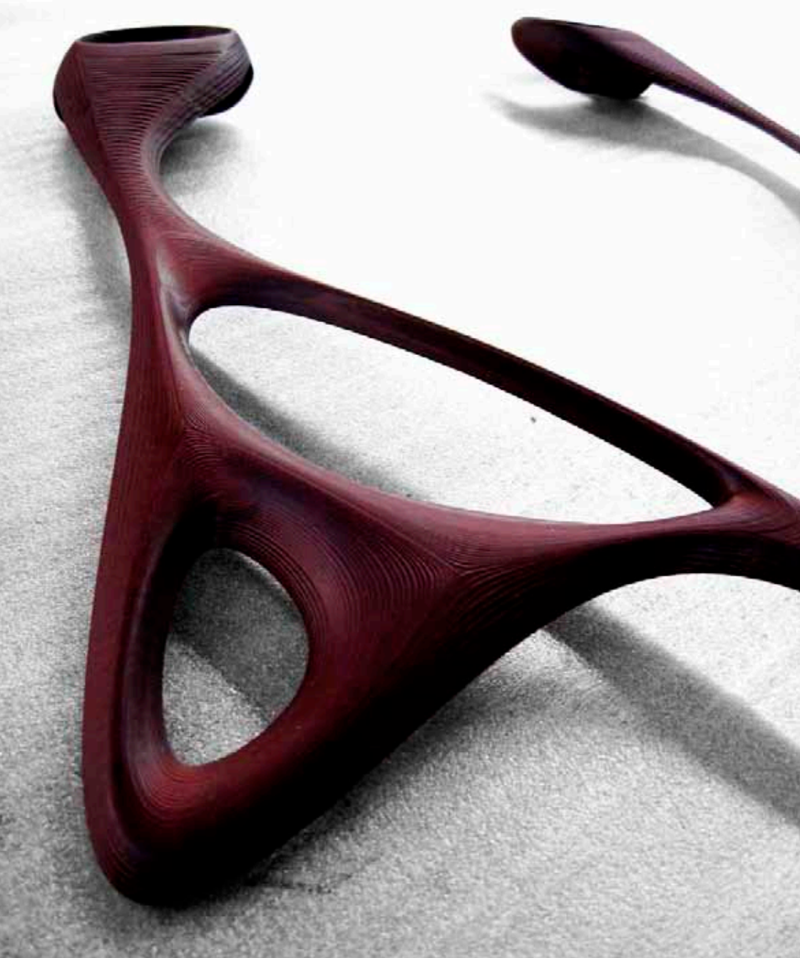
Raw Richlite straps fresh off the CNC Router.
