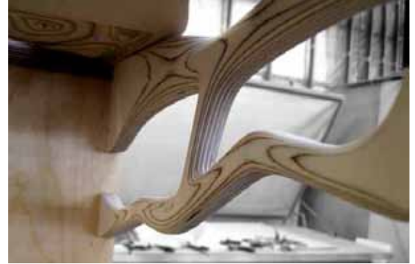
CNC milled arm structure to support the cantilevered desk surface.
