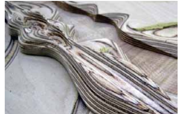
Building up multiple layers of plywood to escape the rigid surface of the sheet material.
