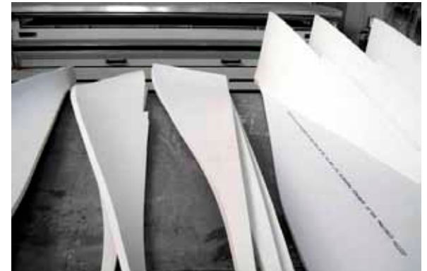
Reusing molds to form small similar surfaces for complex assemblies.
