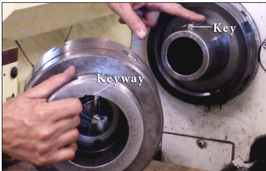
FIGURE 4. THE INSTRUCTOR POINTS AT THE KEY ON THE SPINDLE NOSE. A SLOT CAN BE SEEN ON THE CHUCK, WHICH IS ALSO CALLED THE KEYWAY. THE KEY AND THE KEYWAY NEEDS TO BE ALIGNED TO MOUNT THE CHUCK IN PLACE.
