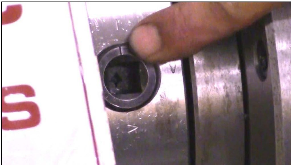
FIGURE 3. AS YOU TIGHTEN THE CAM CLOCKWISE TO LOCK IT IN PLACE, THE LINE ON THE CAM SHOULD BE IN-BETWEEN THE TWO CHEVRON MARKS ON THE SPINDLE.
