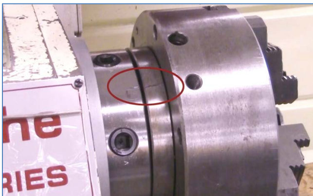
FIGURE 2. CIRCLED ON THE PHOTO ARE THE LINES ON BOTH THE SPINDLE AND THE CHUCK MEETING AT A POINT.
