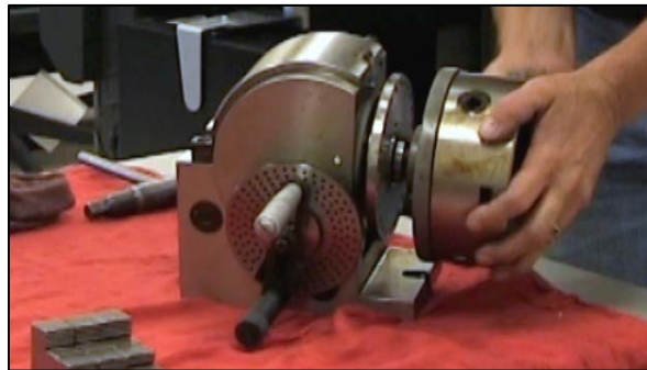
FIGURE 1. THE INSTRUCTOR STARTS THREADING THE 3-JAW CHUCK, WITH A THREADED TAPERED SPINDLE METHOD OF ATTACHMENT, TO AN INDEXING HEAD.
