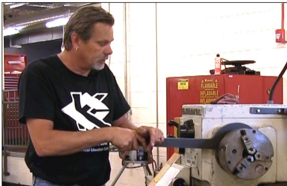
FIGURE 8. THE INSTRUCTOR PREPARING TO TIGHTEN THE THREADED COLLAR AROUND THE CHUCK.
