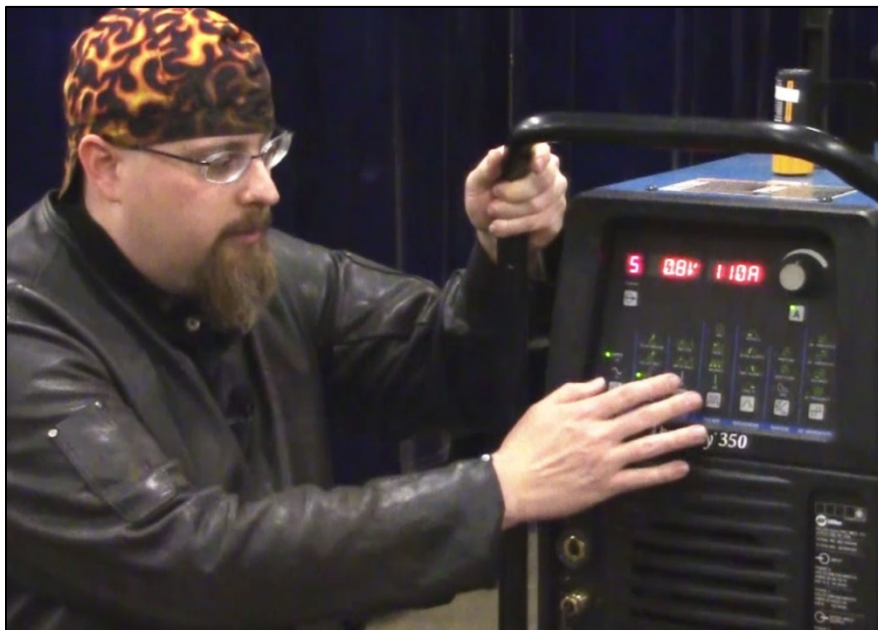
CAPTION 1. THE INSTRUCTOR CHOOSES THE SETTINGS FOR POLARITY, PROCESS, AND OUTPUT.
