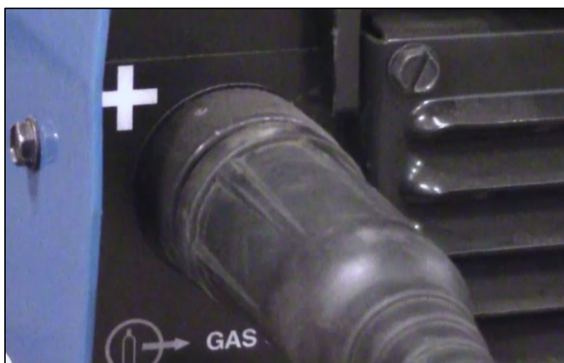
CAPTION 5. IN THE VIDEO, THE INSTRUCTOR USED AN ELECTRODE POSITIVE. THE PHOTO INCLUDES THE CLOSE UP OF THE POSITIVE SYMBOL AND THE ESTABLISHED ELECTRODE POSITIVE CONNECTION.
