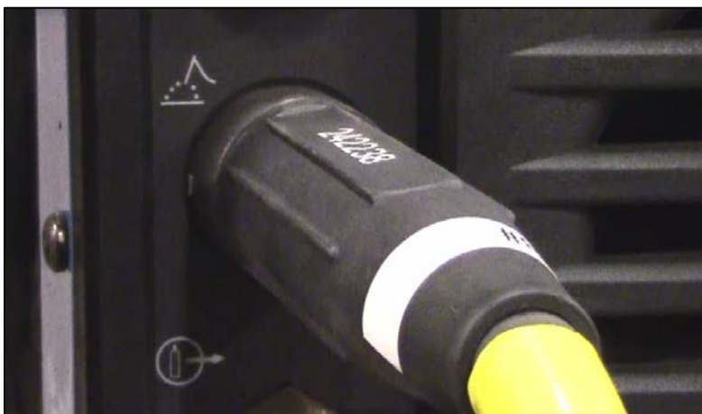
CAPTION 2. THE ELECTRODE LEAD IS CONNECTED. MAKE SURE IT IS PLUGGED INTO THE RIGHT CONNECTION BY LOOKING AT THE SYMBOL BESIDE IT. THE PHOTO INCLUDES A CLOSE-UP OF THE ELECTRODE LEAD SYMBOL.
