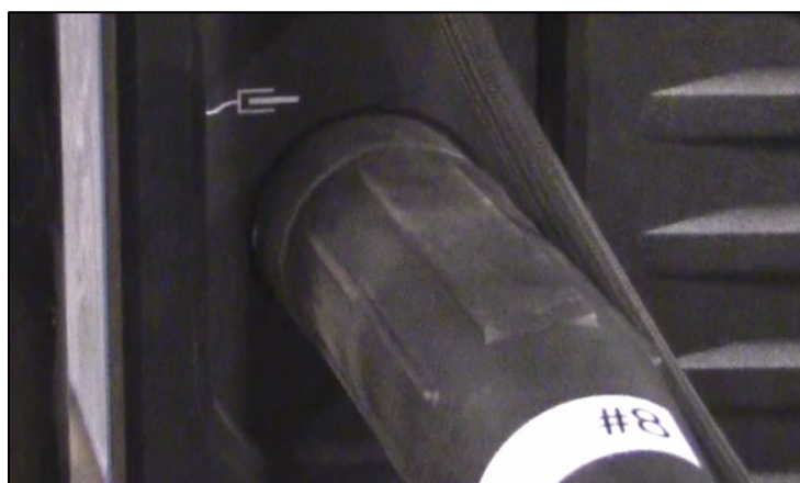
CAPTION 3. THE WORKPIECE CONNECTION WITH A CLOSE-UP OF THE WORKPIECE CONNECTION SYMBOL.
