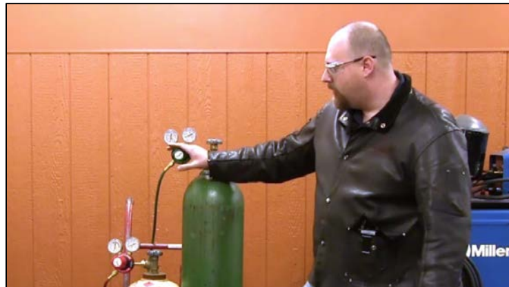
CAPTION 2. THE INSTRUCTOR TURNS THE ADJUSTING SCREW FOR THE OXYGEN TANK OUT. DO THE SAME FOR THE ACETYLENE TANK.
