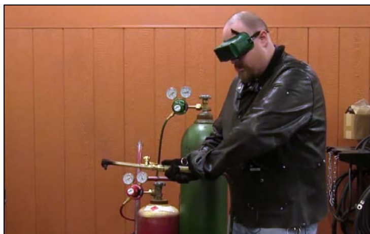
CAPTION 10. THE VALVES ON THE TORCH ARE TURNED OFF.
