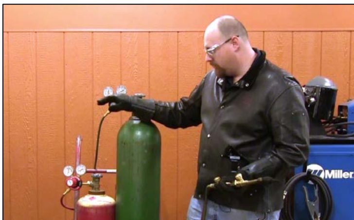
CAPTION 13. THE INSTRUCTOR TURNS THE OXYGEN PRESSURE DOWN WITH THE ADJUSTMENT SCREW.
