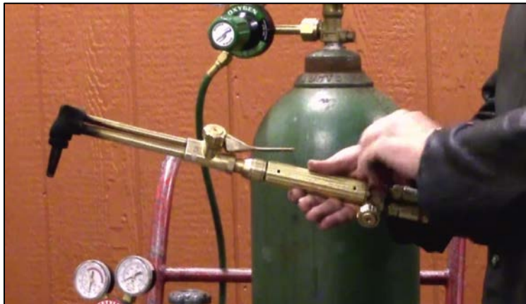
CAPTION 1. THE INSTRUCTOR TURNS THE VALVES ON CUTTING TORCH OFF.
