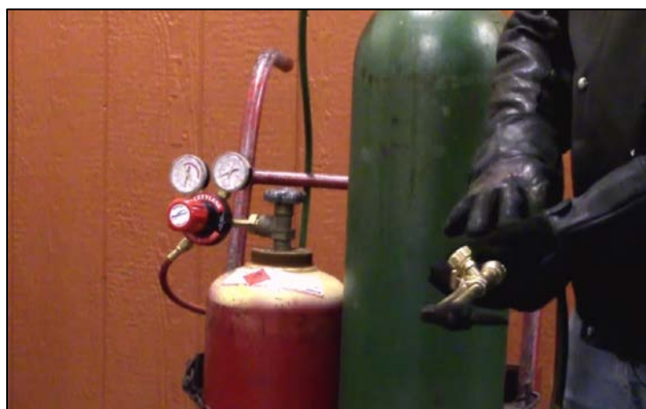
CAPTION 12. THE INSTRUCTOR BLEEDS THE ACETYLENE PRESSURE FIRST. NOTICE THAT THE NEEDLE ON THE PRESSURE GAUGE HAS DROPPED.
