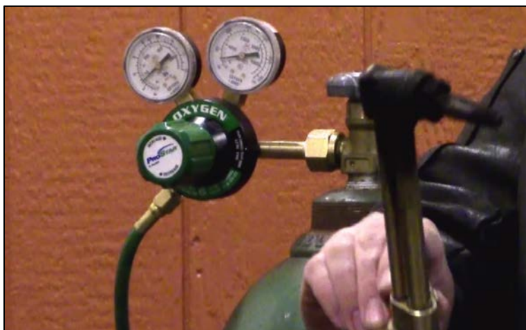
CAPTION 4. THE INSTRUCTOR CHECKS IF OXYGEN IS BEING SUPPLIED TO THE TORCH. NOTICE THAT THE PRESSURE GAUGE NEEDLE HAS MOVED.
