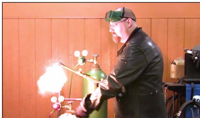
CAPTION 8. THE TORCH IS TURNED ON, AND THE ACETYLENE IS LIT UP.
