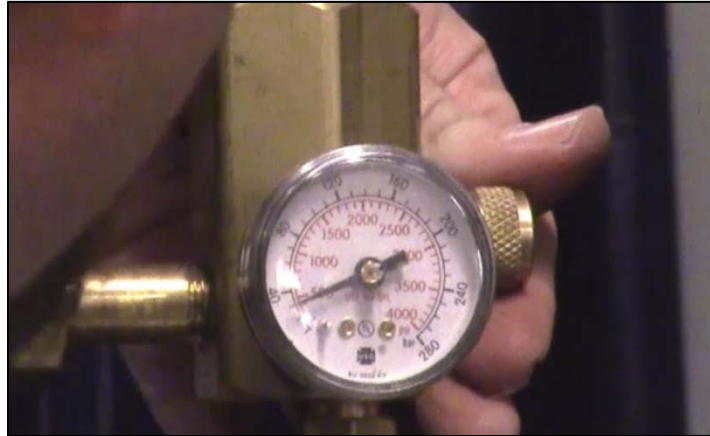
CAPTION 8. THE FLOW RATE OF THE SHIELDING GAS IS SET ON THE GAS TANK.
