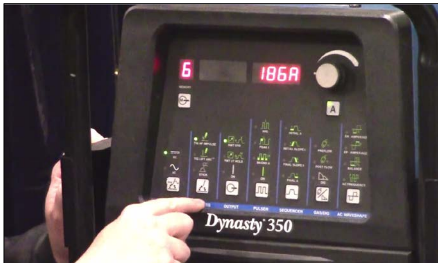
CAPTION 6. A CLOSE-UP OF THE DYNASTY 350. (FROM LEFT TO RIGHT OF THE PHOTO: POLARITY, PROCESS, OUTPUT, PULSER, SEQUENCER, GAS/DIG, AC/WAVE SHAPE)
