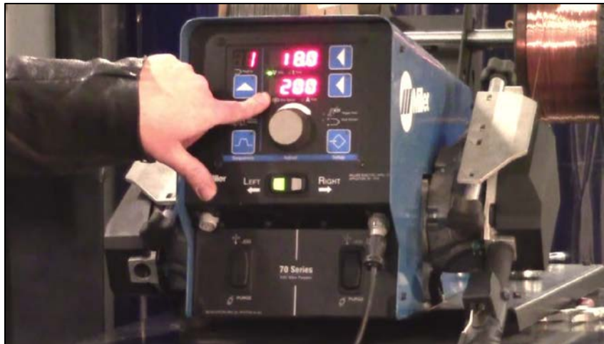
CAPTION 15. THE INSTRUCTOR SETS THE VOLTAGE AND WIRE SPEED.
