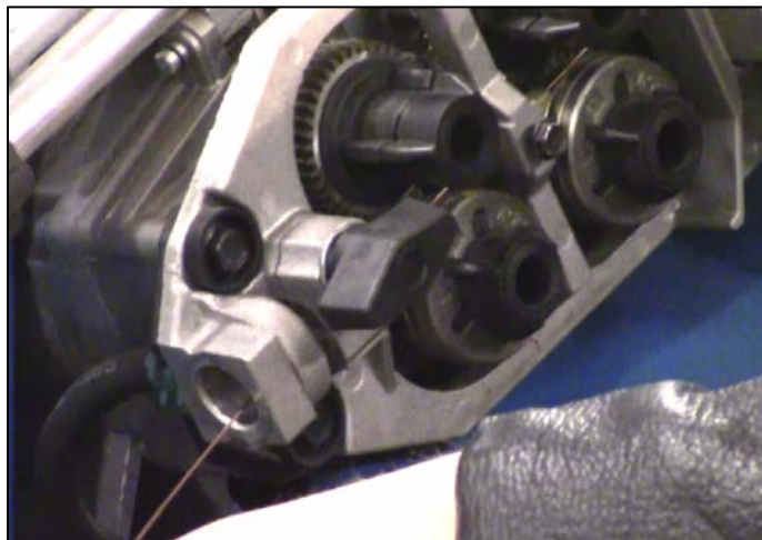
CAPTION 3. THE WIRE IS INSERTED THROUGH THE FEEDER.
