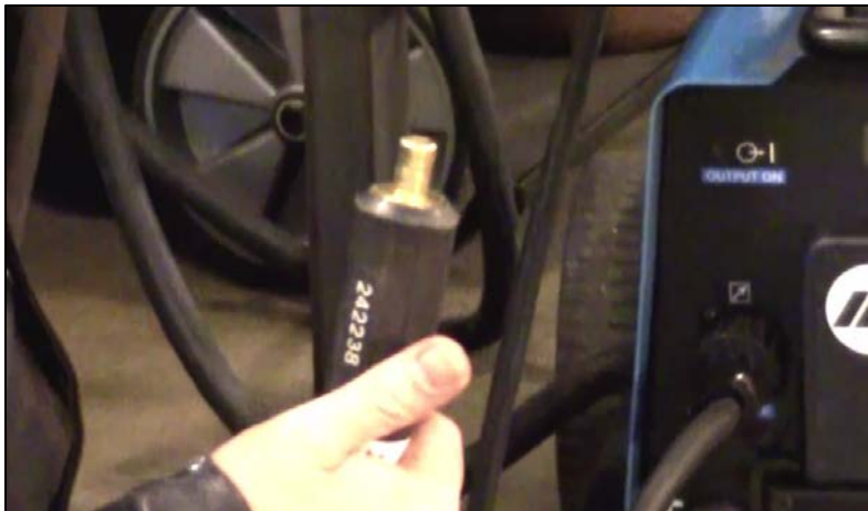
CAPTION 9. THE LEAD CONNECTION SUPPLIES POWER TO THE WIRE FEEDER MACHINE.
