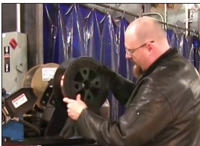
CAPTION 1. FOR THE DEMONSTRATION, THE INSTRUCTOR PLACES A 0.035 ER70S 6 FILLER METAL ON THE WIRE FEEDER.
