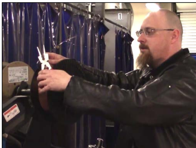
CAPTION 2. CUT THE BENT END OF THE WIRE.
