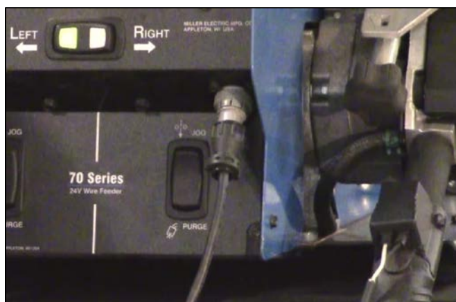
CAPTION 12. THE WIRE IS CONNECTED TO ITS TERMINAL ON THE WIRE FEEDER.
