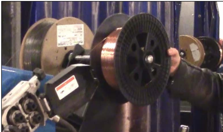
CAPTION 5. THE WIRE SPOOL IS KEPT IN PLACE BY THE CLIP (PLACED RIGHT IN THE MIDDLE OF THE SPOOL).
