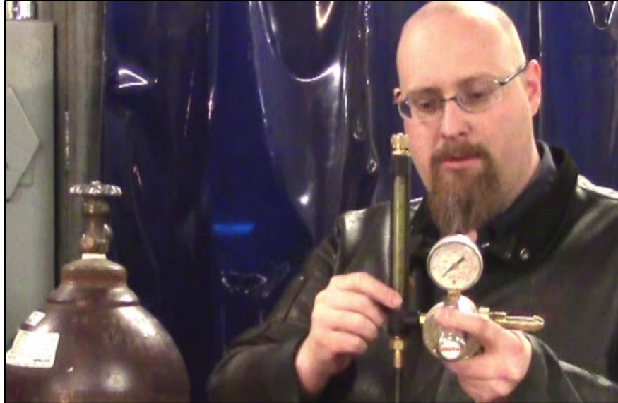
CAPTION 7. THE INSTRUCTOR SHOWS THE FLOW METER THAT WILL BE INSTALLED ON THE GAS CYLINDER.
