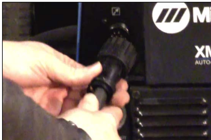
CAPTION 8. THE INSTRUCTOR PLUGS THE 15-PIN CONNECTOR ONTO THE XMT 350 MPA MACHINE.
