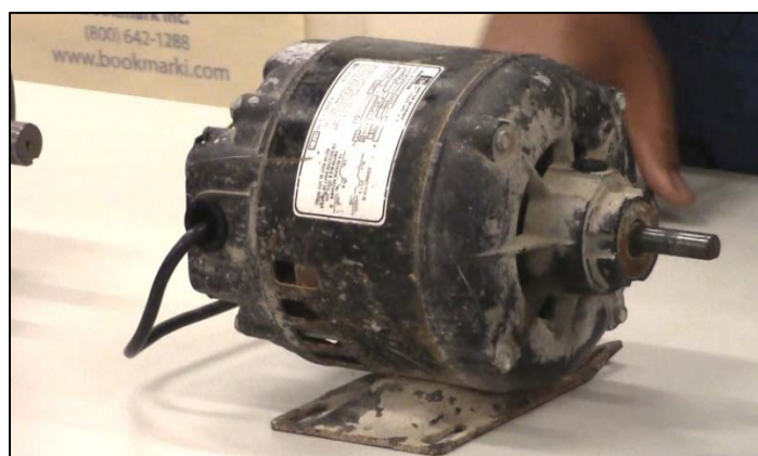
FIGURE 2. AN EXAMPLE OF A SPLIT-PHASE MOTOR WITH A CORD AND PLUG CONNECTION.
