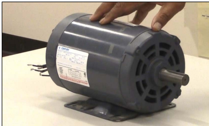
FIGURE 1. THE INSTRUCTOR SHOWS AN EXAMPLE OF AN INDUCTION MOTOR. THIS IS A SINGLE PHASE INDUCTION MOTOR WITH DUAL VOLTAGE.
