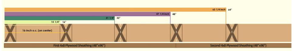
CAPTION 1 AN ILLUSTRATION OF WHAT THE MEASUREMENTS ARE FOR 16-INCH ON CENTER WALL LAYOUT, BASED ON THE VIDEO WALL LAYOUT. IN THE ILLUSTRATION ABOVE, A 4X8 PLYWOOD SHEATHING ENDS ON A STUD. THE STUD PROVIDES A SURFACE AREA TO NAIL THE PLYWOOD SHEATHING ON.
