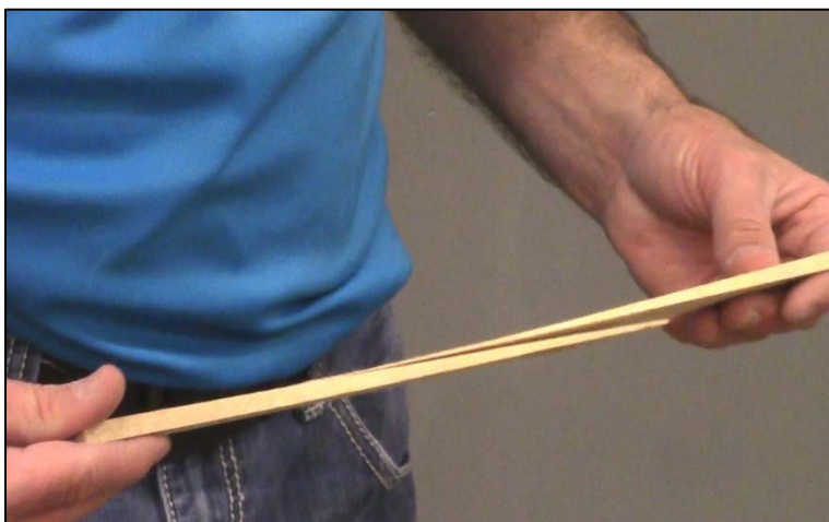
CAPTION 4. THE INSTRUCTOR SHOWS 2 SHIMS. SHIMS CAN BE LAYERED TOGETHER TO FIT IN A GAP.
