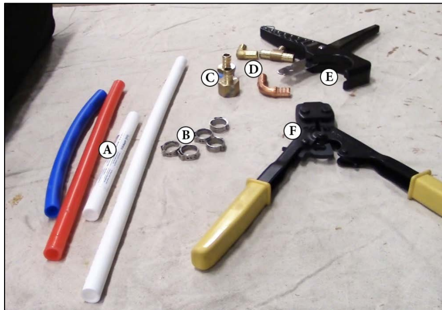
CAPTION 10. A PHOTO OF THE MATERIALS USED IN THE VIDEO FOR INSTALLING A FITTING ON A PEX SUPPLY LINE. EACH ITEM HAS A CORRESPONDING ALPHABET LABEL.
