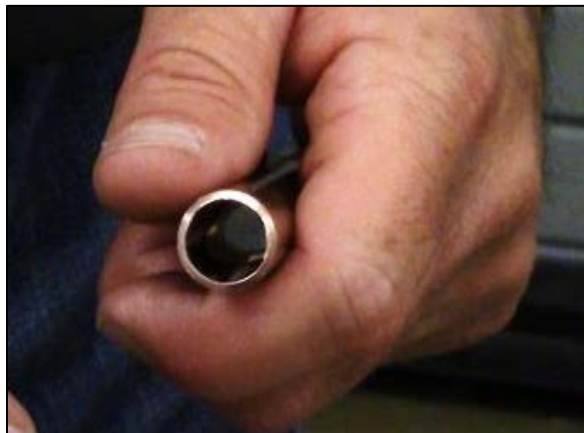
CAPTION 4. A CLOSE-UP OF THE CUT COPPER PIPE
