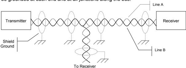
The transmitting source output impedance should be 75  $\Omega$   $\pm$  5  $\Omega$  divided equally between Line A and Line B. This balanced output should closely match the impedance of the cable. The receiving sink must have an effective input impedance of 8k  $\Omega$  minimum.
