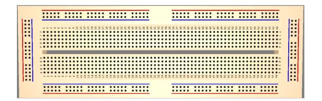
If you could see inside the breadboard, it would look like the image in the second figure. This image shows how the holes on the breadboard are connected on the inside. Any hole that lies on the same line (or wire) are said to be electrically common. Any connection along that same set of holes is the same connection. The areas that are outlined with red and blue stripes are bus lines. The area in the center is where circuits are built.
