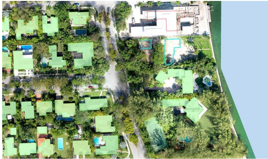
Figure 9. Aerial image captured with drones and footprints as present in the City of Miami GIS data.
