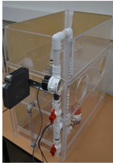
Level Control of Upper Tank with Multiple Drains and Feedback from Level Sensor
