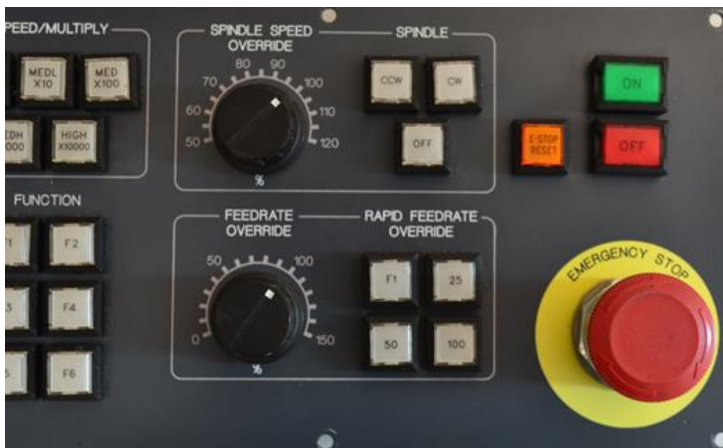
Fig. 17-26b HMI Panel for Series-9 A-B Multi-Axis Motion System (rt side)
