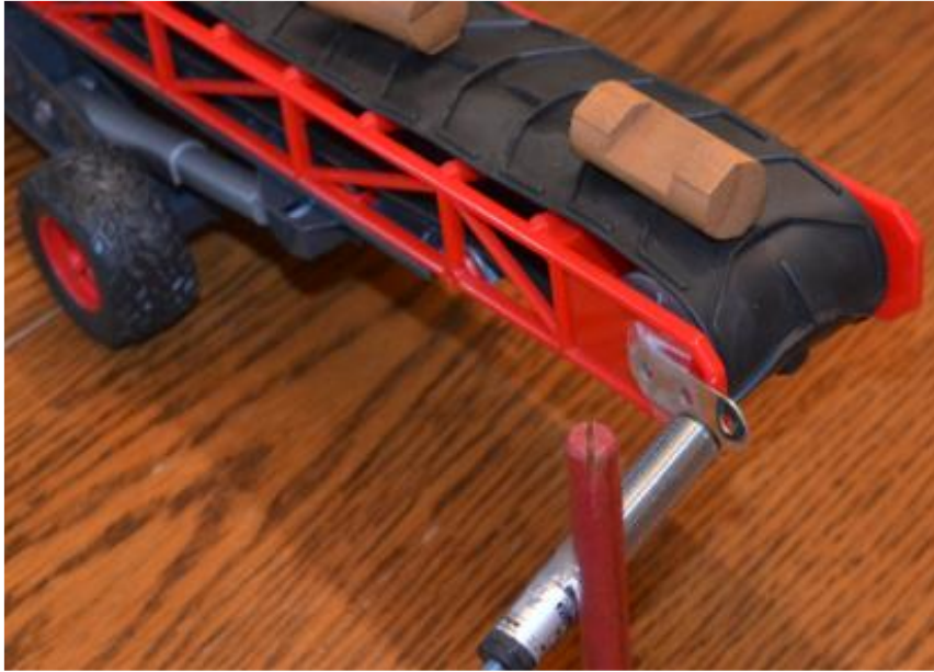
Fig. 7-40 A zero speed switch is built from a rotating metal piece attached to the shaft and a proximity switch
