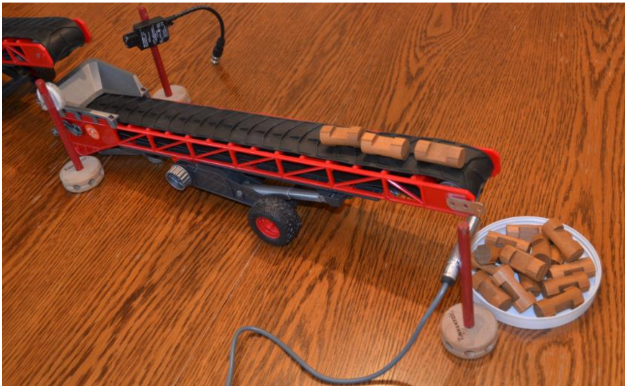
Fig. 7-44b Conveyor Problem with Material Tracking
