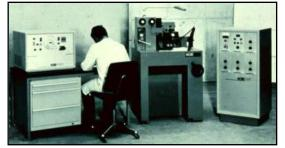
immediately began to replace RC generators. While many different makes and models of sinkers evolved over the years, there were no big breakthroughs in EDM until 1969 when Prof. Bernd Schumacher of AGIE announced the development of the first wire EDM, the AGIECUT DEM-15, at left. (No, that is not Dr. Schumacher)
