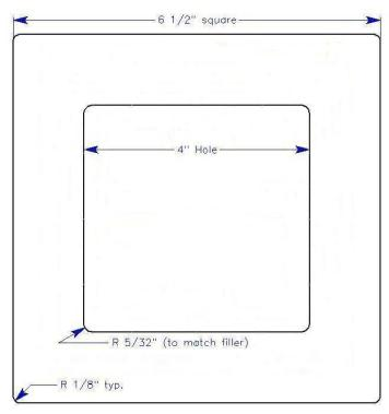
(2) Next layout the filler and doubler in accordance with the drawing below.
