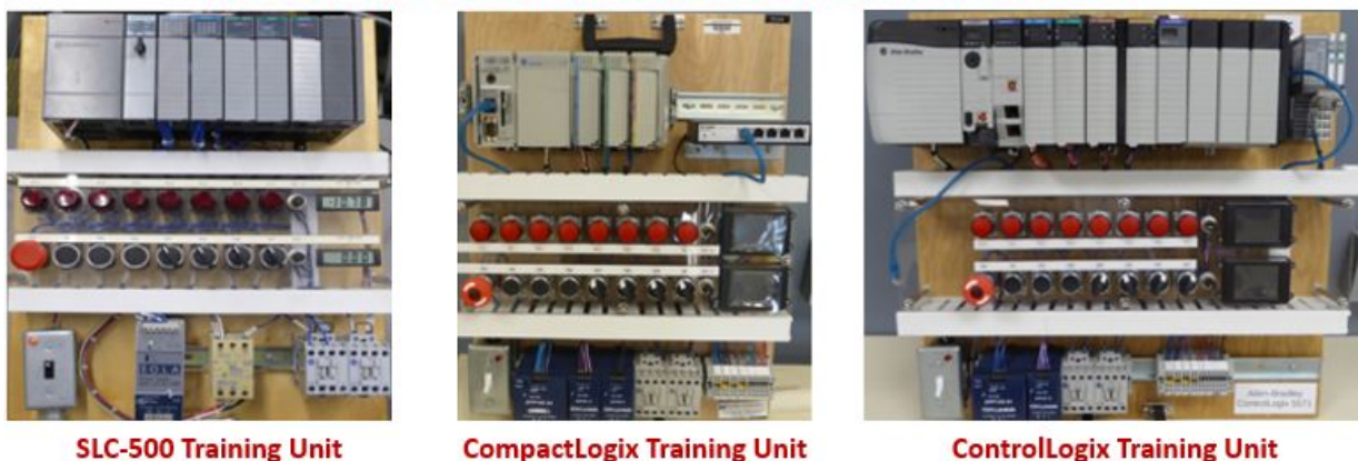
Figure 1. The PLC Hardware Simulators.
