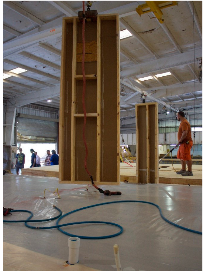
FIGURE 1.29, 1.30: THE SIDE WALL IS BUILT IN THE OFFLINE STATION AND THEN SET ON THE ONLINE PRODUCTION LINE.
