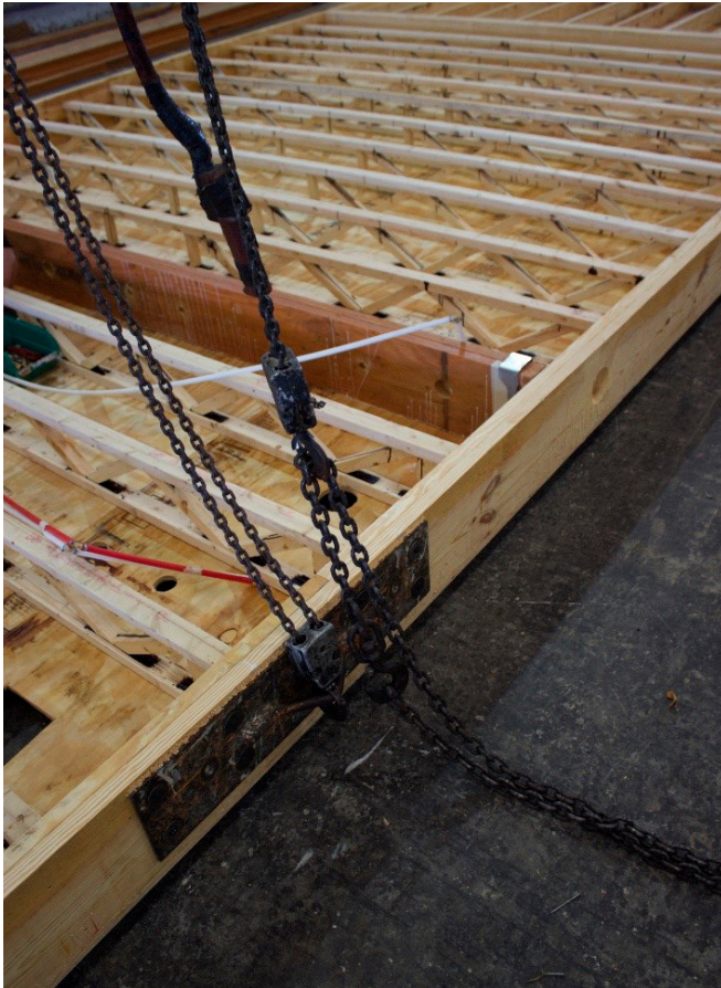
FIGURE 1.29, 1.30: THE SIDE WALL IS BUILT IN THE OFFLINE STATION AND THEN SET ON THE ONLINE PRODUCTION LINE.
