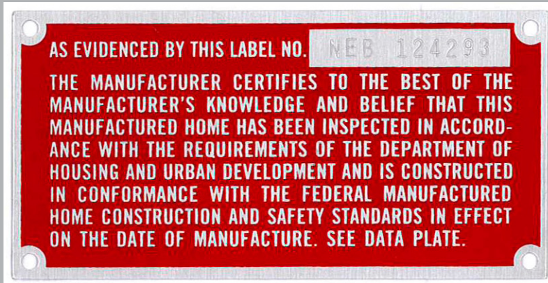
FIGURE 2.8 MANUFACTURED HUD HOMES ARE IDENTIFIED BY A HUD CODE LABEL THAT IS AFFIXED TO THE OUTSIDE OF THE HOME. IT IS A LIGHT METAL AND IS USUALLY A REDDISH COLOR AND WILL ALWAYS HAVE THE TERM "HOUSING AND URBAN DEVELOPMENT" WITHIN THE TEXT. THE CODE LABEL ATTESTS THAT THE HOME HAS BEEN MANUFACTURED USING AN EFFECTIVE QUALITY CONTROL PROGRAM.
