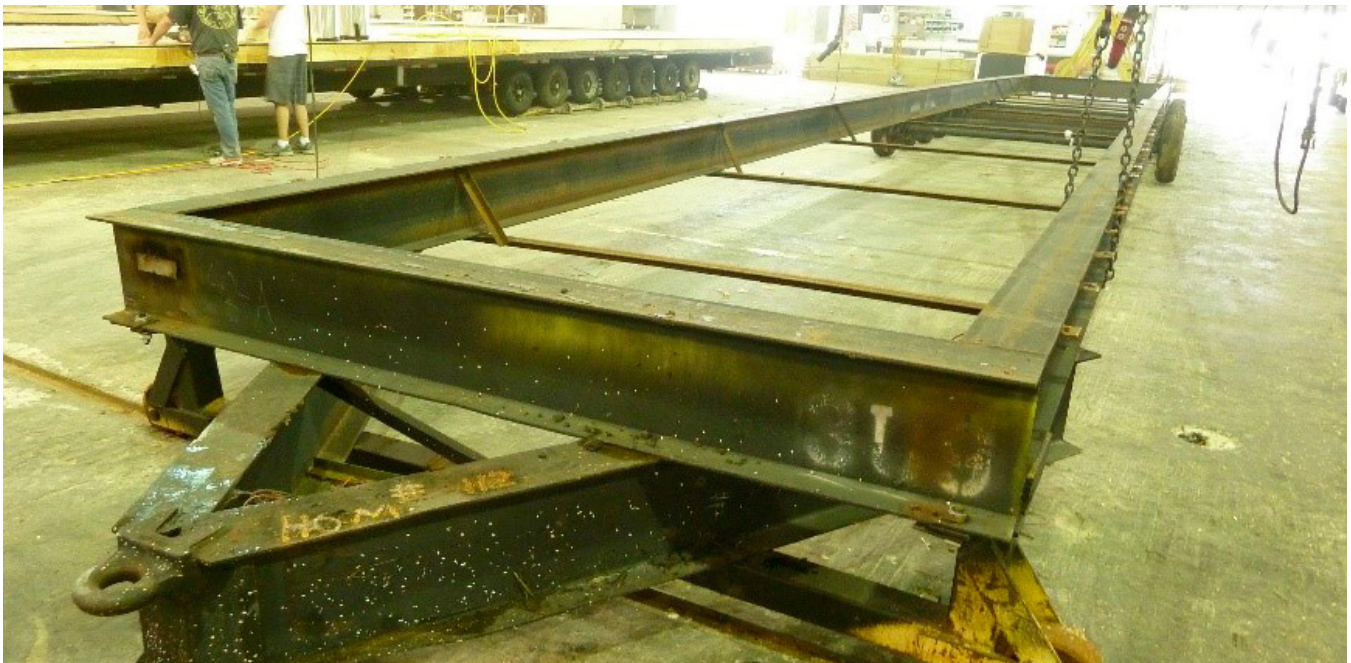
FIGURE 1.7: CHASSIS IS BUILT AND MOVED ON RAIL TO FACILITATE FLOW ON THE ONLINE PRODUCTION LINE. ALTHOUGH THE CHASSIS IN THIS PHOTO DOES NOT USE OUTRIGGERS, SOME CHASSIS WILL REQUIRE THEM FOR THE TYPE OF HOME THEY ARE SUPPORTING AND TRANSPORTING.
