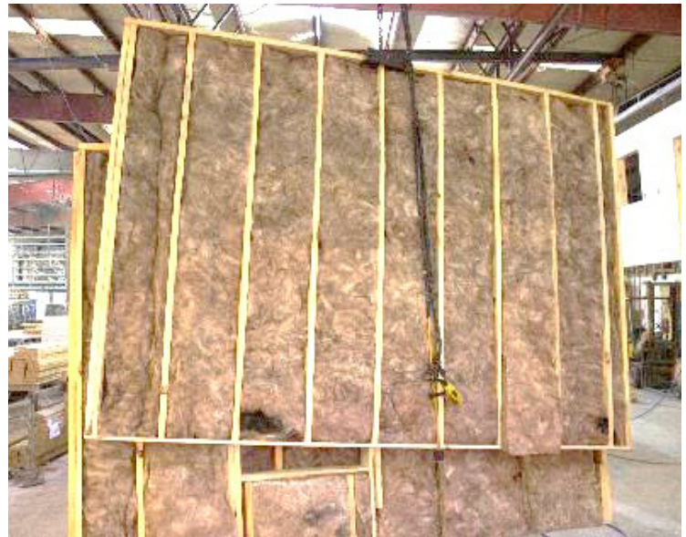
FIGURE 1.26, 1.27 AND 1.28: THE INDIVIDUAL WALLS ARE BUILT AND STORED, READY TO BE LIFTED AND USED IN THE NEXT STATION, THE SET WALL STATION.
