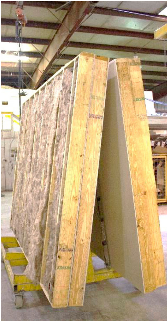
FIGURE 1.26, 1.27 AND 1.28: THE INDIVIDUAL WALLS ARE BUILT AND STORED, READY TO BE LIFTED AND USED IN THE NEXT STATION, THE SET WALL STATION.
