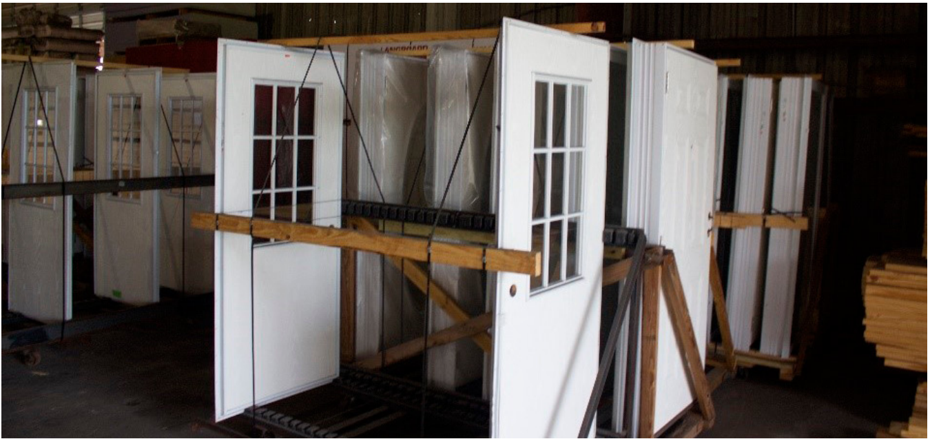
FIGURE 1.53: PRE-MADE DOORS ARE STORED AND READY TO BE INSTALLED DURING THE ON-LINE PRODUCTION PROCESS.
