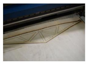
6. Leave cut pieces in the machine. Invert the line widths (change outer to 3 pt., inner to hairline). Set up machine for vector engraving to add interior details. Add to both sides. Check the vector engraving settings.
