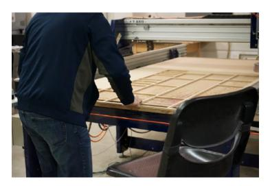
2. Secure MDF to the table with a drill and construction screws. To do this, screw the corners to the bed of the machine.
