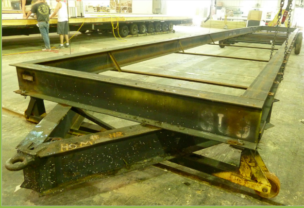
FIGURE 2.11: A TYPICAL CHASSIS READY TO BE PAIRED WITH THE UNIT FLOORING
