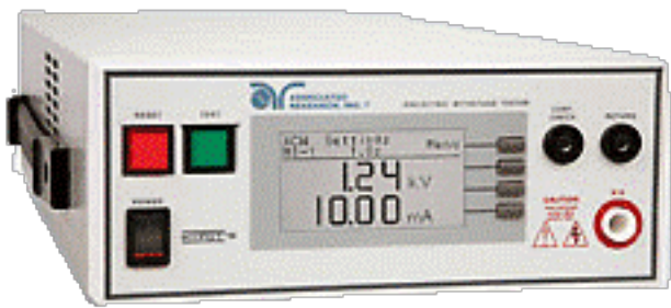
FIGURE 2.37 DIELECTRIC TESTER APPLIES THE NECESSARY VOLTAGES TO THE ELECTRICAL SYSTEM AND MONITORS LEAKAGE CURRENT.
