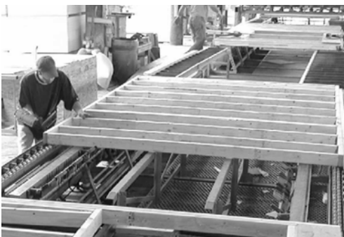
(CLOCKWISE FROM ABOVE)FIGURE 3.2 WALL PANELS ARE FRAMED USING PRECUT COMPONENTS. (SOURCE: U.S. DEPARTMENT OF HOUSING AND URBAN DEVELOPMENT) FIGURE 3.3 APPLICATION OF SHEATHING PANELS TO FRAMING. (SOURCE: U.S. DEPARTMENT OF HOUSING AND URBAN DEVELOPMENT) FIGURE 3.4 A ROUTER IS USED TO CREATE PANEL OPENINGS. (SOURCE: U.S. DEPARTMENT OF HOUSING AND URBAN DEVELOPMENT) FIGURE 3.5 FINISHED PANELS ARE HOISTED FROM THE PRODUCTION LINE AND STACKED WITH OTHER PANELS FOR DELIVERY TO THE JOBSITE. (SOURCE: U.S. DEPARTMENT OF HOUSING AND URBAN DEVELOPMENT)
