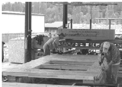
(CLOCKWISE FROM ABOVE)FIGURE 3.2 WALL PANELS ARE FRAMED USING PRECUT COMPONENTS. (SOURCE: U.S. DEPARTMENT OF HOUSING AND URBAN DEVELOPMENT) FIGURE 3.3 APPLICATION OF SHEATHING PANELS TO FRAMING. (SOURCE: U.S. DEPARTMENT OF HOUSING AND URBAN DEVELOPMENT) FIGURE 3.4 A ROUTER IS USED TO CREATE PANEL OPENINGS. (SOURCE: U.S. DEPARTMENT OF HOUSING AND URBAN DEVELOPMENT) FIGURE 3.5 FINISHED PANELS ARE HOISTED FROM THE PRODUCTION LINE AND STACKED WITH OTHER PANELS FOR DELIVERY TO THE JOBSITE. (SOURCE: U.S. DEPARTMENT OF HOUSING AND URBAN DEVELOPMENT)
