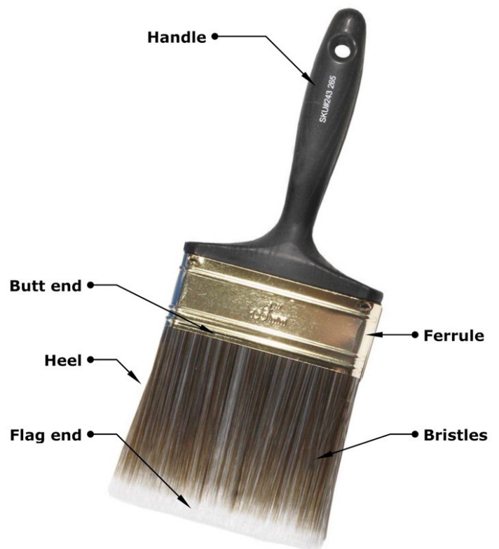
FIGURE 2.30 TYPICAL PAINT BRUSHES ARE COMPOSED OF BRISTLES, A HEEL, A FERRULE, AND A HANDLE.
