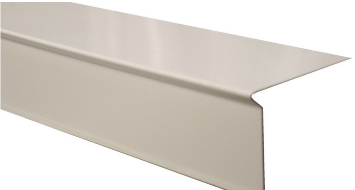
FIGURE 2.5 DRIP EDGE FLASHING IS USED ALONG THE ROOF EDGES TO AVOID WATER LEAKAGE (SOURCE: LOWE'S COMPANIES)
