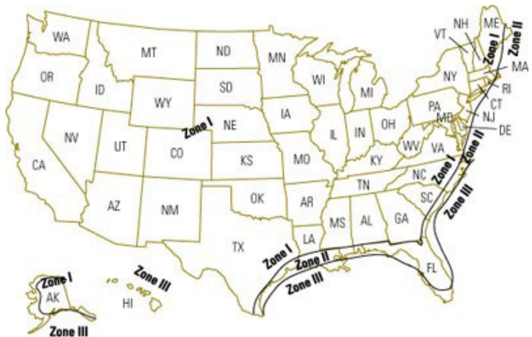
FIGURE 1.6 THERE ARE THREE WIND ZONES IN THE HUD CODE, WITH WIND ZONE III DESIGNATING THE HIGHEST WIND VELOCITIES. THE HIGHER THE WIND ZONE, THE MORE STRINGENT THE REQUIREMENTS FOR CONNECTING THE HOME AND IT COMPONENTS TOGETHER AND TO THE GROUND.
