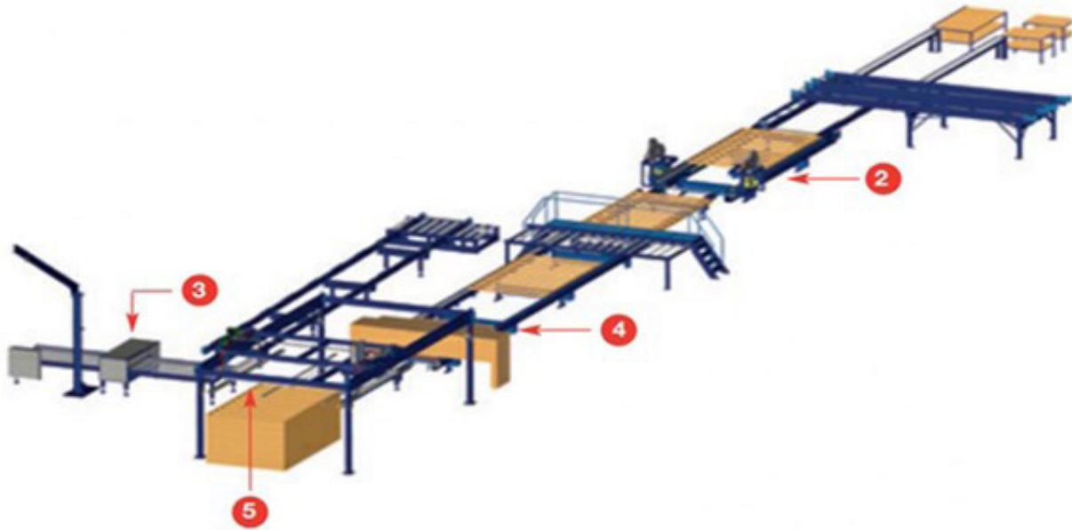
FIGURE 3.7 - SCHEMATIC EXAMPLE OF THE MITEK PANELIZED PRODUCTION LINE. THIS AUTOMATED PRODUCTION LINE USES SOFTWARE CALLED EFRAME, WHICH DESIGNS ALL THE WOOD ELEMENTS. THE PROCESS STARTS WITH THE COMPONENT PROCESSING CENTER, WHERE THE PROPER MATERIAL MUST BE LOADED IN THE MACHINE. AFTER THAT, DIMENSIONAL LUMBER IS FED TO THE POWER FRAMER (2) WHERE PANELS MOVE THROUGH FOUR HIGH-PRODUCTION NAIL GUNS. A TWIN-AXIS SHEATHING SAW (3) CUTS THE SHEATHING IN X AND Y AXES SIMULTANEOUSLY. A POWER SQUARING AND SHEATHING STATION (4) ATTACHES THE SHEATHING TO THE TOP AND BOTTOM PLATES. FINALLY, A SMART CRANE STACKER (5) AUTOMATICALLY STACKS FULL LEVELS OF 16' WALLS AND PROVIDES BUILT-IN FORK POCKETS FOR EASY TRANSPORT OF COMPLETED PANELS. (SOURCE: MITEK)
