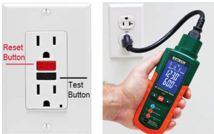
FIGURE 2.39 - GFCI TRIPPING DEVICE (LEFT) AND GFCI CIRCUIT TESTER (RIGHT) ARE USED IN OPERATIONAL TESTS.
