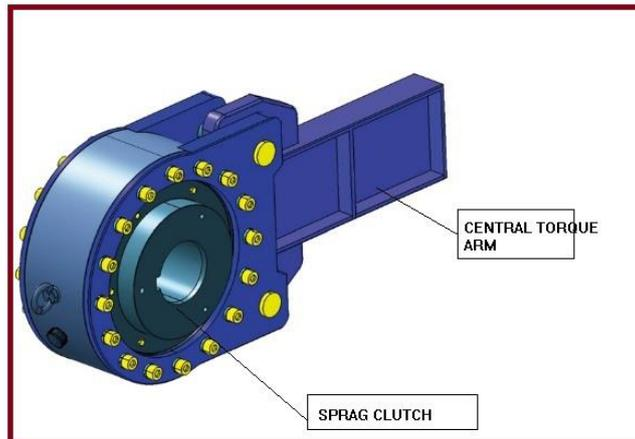
**Caption:** In the case of an inclined conveyor, the function of the backstop is to keep the conveyor loaded with gravel from running backward if a power failure occurs.
