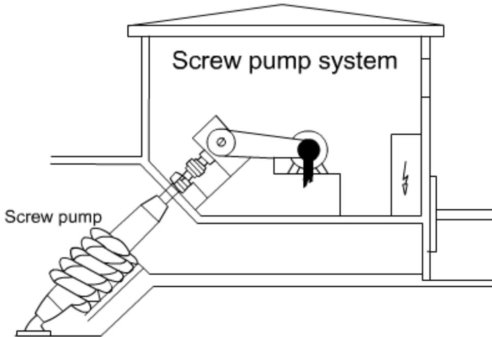
**Caption:** Industrial centrifugal pumps and screw pumps sometimes use backstops to prevent reverse rotation when the motor is stopped and the pumpage may tend to run back through the pump.
