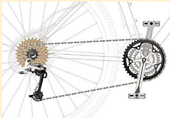
Let's take an example of a bicycle. With its freewheel mechanism, the rider can pedal to make the rear wheel turn. However, the wheel does not make the pedals turn. This configuration allows the rider to coast downhill without pedaling.
