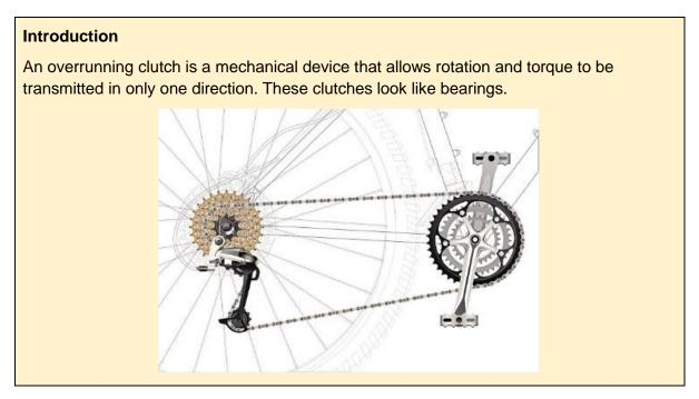
Let's take an example of a bicycle. With its freewheel mechanism, the rider can pedal to make the rear wheel turn. However, the wheel does not make the pedals turn. This configuration allows the rider to coast downhill without pedaling.
