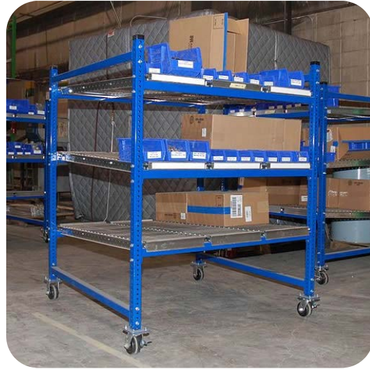
Figure 44. Gravity flow rack. By Markj52 (Own work) [CC BY-SA 3.0 or GFDL], via Wikimedia Commons.
