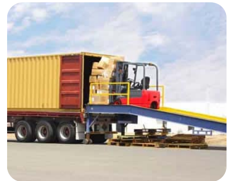
Figure 58. Mobile ramp in use. Developed by LINC'S in Supply Chain Management Consortium.
