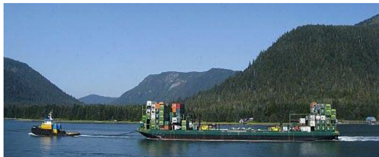
Figure 15: Tugboat moving barge for loading onto LASH. By Christine [CC BY-SA 2.0], via Wikimedia Commons.
