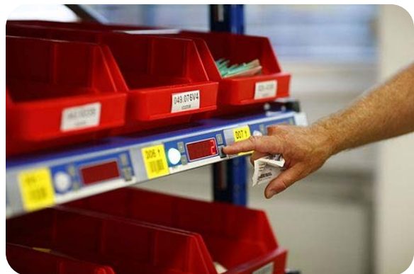
Figure 33. Pick-by-light. By KBS Industrieelektronik GmbH (Own work) [CC BY-SA 3.0], via Wikimedia Commons
